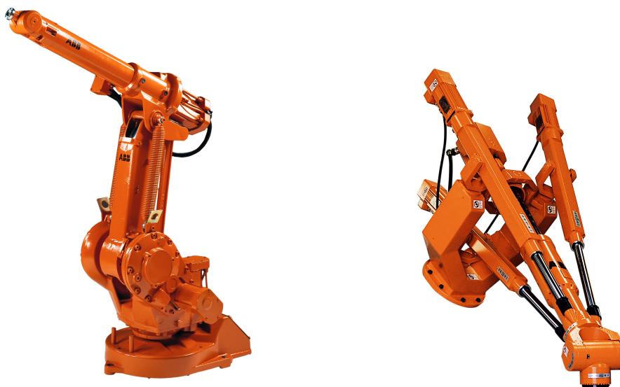
Figure 1.1: A serial manipulator (left), the ABB IRB1400, and a parallel manipulator (right), the ABB IRB940Tricept. Photos courtesy of ABB Robotics.
